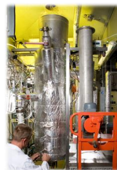
Figure 2: 5 kW th BFB facility at ECN.
