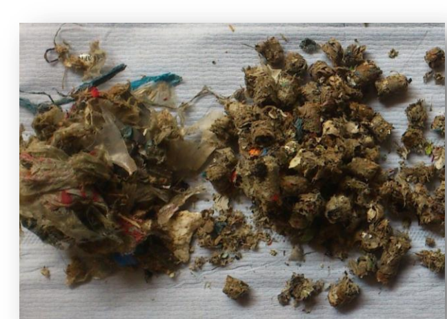
Paper rejects: raw (left), and after 8 mm pelletization (right).
