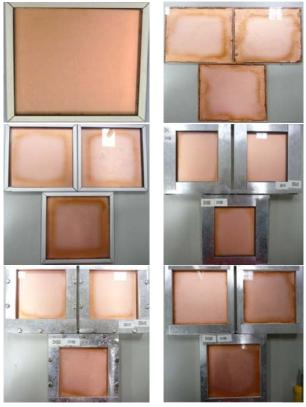
**Figure 4:** Visual appearance of tested coupons with alternative edge sealants after 1000 hours in DH. Upper left: sample before DH test. Upper right: without edge sealant. Middle right: double side adhesive tape (reference). Middle right: U-profile. Below left: "O"-ring and below right: sponge rubber
