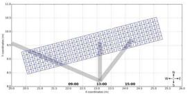
Figure 8: Graphic representation of the look up table for specific time and date produced by the shading model
