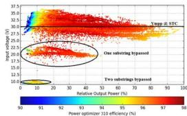
**Figure 8**: Relation of input voltage with efficiency and power output during 5 months of operation under clear and partially shaded conditions. The PO310 can operate even with one illuminated substring and thus track the global maximum even at extreme shading conditions.
