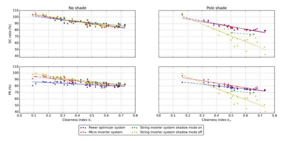
**Figure 9:** Daily calculated PR and DC ratio versus average clearness index of the day for unshaded and partially shaded operation of the three systems with a pole shading 1-2% of the total PV system surface. Data presented at the graph are calculated during spring months.
