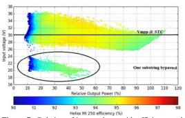
**Figure 7**:. Relation of input voltage with efficiency and power output during 5 months of operation under clear and partially shaded conditions. The micro inverter includes a hybrid P&O MPPT algorithm which can track global maximum by performing regularly IV scans.
