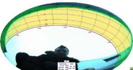
**Figure 4**: Skyline picture shoot from the micro inverter system facing south-east. Clearly visible is the wall on the south side of the solar panels highlighted with green colour. Additionally the east and west neighboring building can be seen. An average solar access of 83% has been calculated for the specific location.
