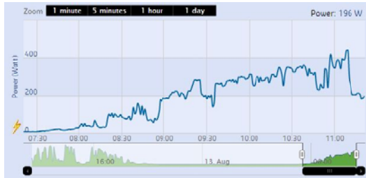
Figure 8: AC power measured per second, possibly averaged in various relevant time scales (1 minute, 5 minute, 1 hour, 1 day).
