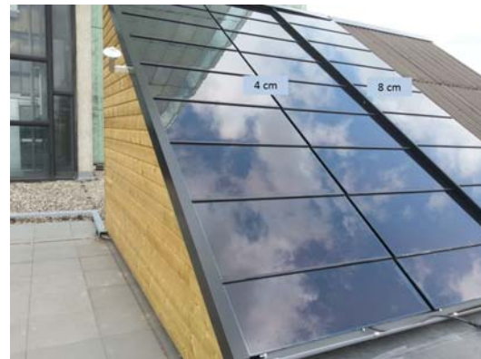
Figure 1: A dummy house with a typical Dutch attic. Three rows are used for experiments with a new BIPV-product that is combining thermal insulation and CdTe PV-panels. The insets shows the air gap depth, which is varied between 4 and 8 cm to investigate thermal effects.
