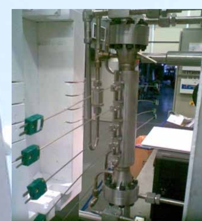
tube-in-tube reactor (inner tube filled with the activated carbon, oil coolant flow between inner and outer tube)
