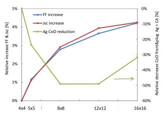
Figure. 5. Calculated relative FF and Jsc variations as a function of the number of vias for MWT-HJ cells. The cost of ownership (CoO) reduction of the front contact silver including plug and conductive adhesive (CA) is also calculated (right axis).
