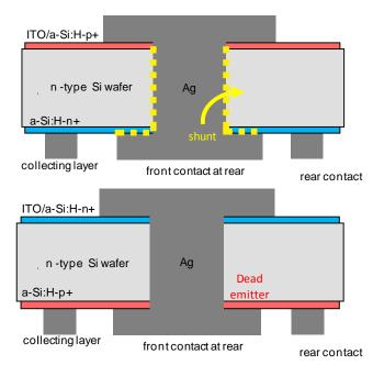
Figure 2. Structure of a front (top) and rear (bottom) emitter MWT-HJ solar cell.
