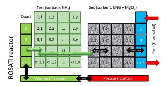
Figure 4: Definition of the calculation grid of the SOSYMO model.
