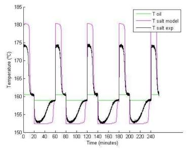
Figure 7: The relation between temperature of thermal oil (measured = green) and salt (measured = black, calculated = pink) as a function of time.
