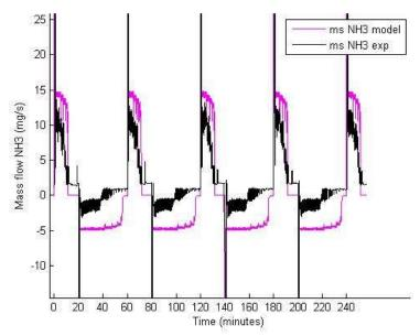
Figure 8: The measured (black) and calculated (pink) mass flow of NH<sub>3</sub> as a function of time.
