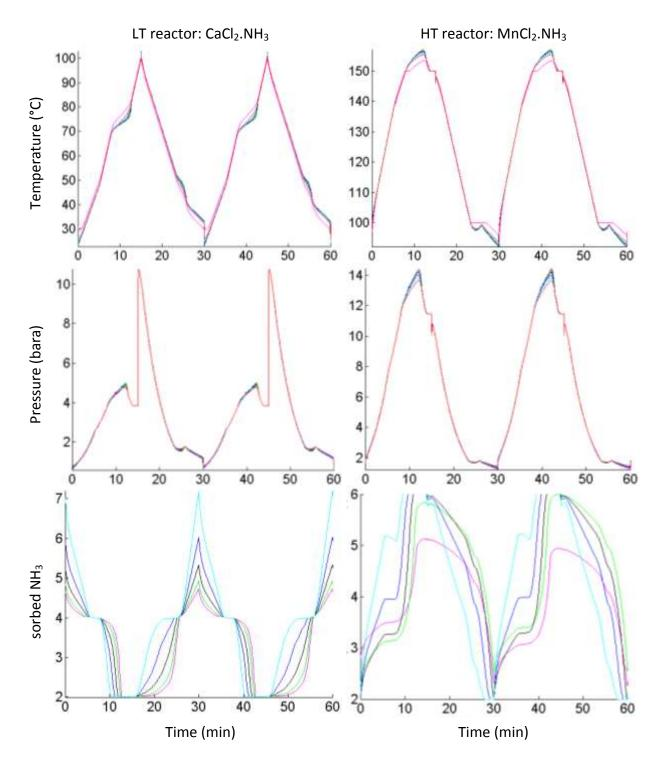
Figure 6: Model calculations of sorbent temperature, pressure and amount of NH<sub>3</sub> sorbed as a function of time for a system with 1 MW heat output
