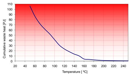
Figure 1: Amount of waste heat actively disposed in the Dutch refinery and chemical industry as a function of the waste heat temperature.
