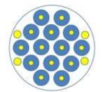
Figure 3: Schematic representation of lab scale shell-n-tube type reactor with blue the sorbent material and in yellow the open gas volume – allowing the sorbate to flow through the tubes and the white represents the heat transferring medium.
