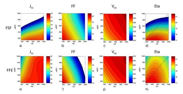
Figure 4: Modelled performance comparison of the IBC cell with FSF and FFE. The IV parameters  $J_{sc}$ , FF,  $V_{oc}$  and cell efficiency are presented as a function of emitter and BSF width. The values shown are based on the unit cell and are thus half-widths and are expressed in  $\mu m$ . The diagonal dashed line in d) and h) indicates cell designs with equal widths for emitter and BSF.
