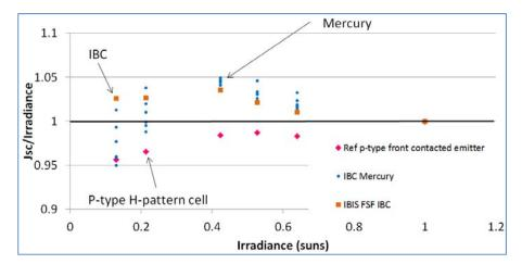
Figure 8: linearity of Mercury IBC cells. The ratio  $J_{sc}/J_{sc}(1-sun)$  was plotted as function of the irradiance for 3 cell types: FSF-IBC, FFE-IBC, p-type front junction.
