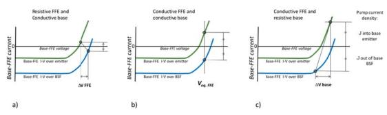
Figure 3: The qualitative illustration on the mechanism of the pumping effect in the FFE showing the IV-curves of base-FFE junction above BSF and emitter for 3 cases of resistivity of FFE and wafer in order of increase pump current. The magnitude of the pump current I and the relevant voltage drop affecting it is illustrated in each case.
