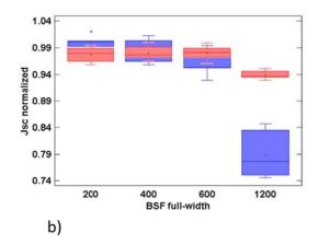
Figure 6: a) Simulated and experimental values for  $J_{sc}$  of the Mercury cells with different wafer resistivity and different BSF full widths. The emitter width is fixed to 1600  $\mu$ m b) Normalized short-circuit densities as a function of BSF width measured on small-sized IBC cells (~13 cm<sup>2</sup>) with FSF (blue) and FFE (red).
