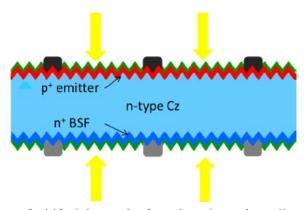
Figure 7: Cross-section of a bifacial n-pasha front-junction solar cell.
