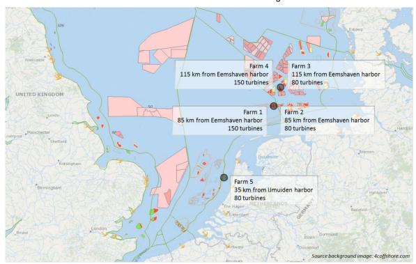
Figure 5: The five wind farms considered for the comparison of O&M concepts for future faroffshore sites [11].
