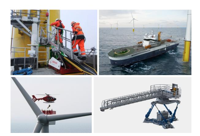
Figure 3: Examples of alternative access systems. In anti-clockwise direction starting top left: the MaXccess [4] system for enhancing workboat workability, helicopter transfer [5], the Z-Bridge access system [6] placed on the Damen W2W vessel [7] and Ampelmann [8] compensated access gangway.
