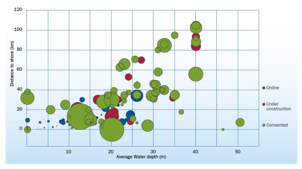
Figure 1: Graph illustrating the farm size, distance to shore and average water depth for offshore wind farms currently being online, under construction and consented [1].
