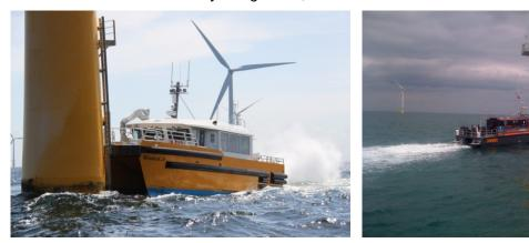
Figure 2: Examples of catamaran-like workboat access vessels: the WindCat MKIII on the left [2] and the CTruk 20T on the right [3].
