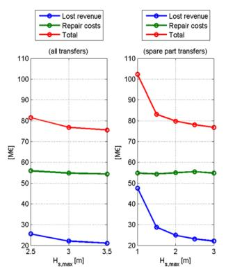
Figure 7: Analysis of the influence of the wave height limit for transfers via a compensated access gangway on the wind farm lost revenues and cost of repair.
