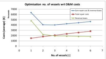
Figure 4: The OMCE-Calculator: ECN's software for advanced OPEX cost modelling. On the left an example of its GUI, on the right an example to find the optimal number of access vessels.
