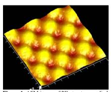
Figure 1: AFM image of 2D structure applied: period  $\approx 1$  µm; height  $\approx 300$  nm
