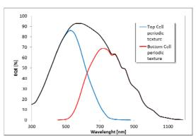
**Figure 2:** EQEs of tandem cell with 300 nm thick top and 1000 nm thick bottom cells on steel substrate with UV lacquer embossed with periodic texture.
