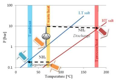
Figure 3: Thermodynamic cycle of the hybrid heat pump type II configuration.
