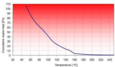
Figure 1: Amount of waste heat actively disposed in the Dutch refinery and chemical industry as a function of waste heat temperature.
