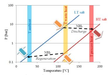
Figure 2: Thermodynamic cycle of the heat-driven heat pump type II configuration.
