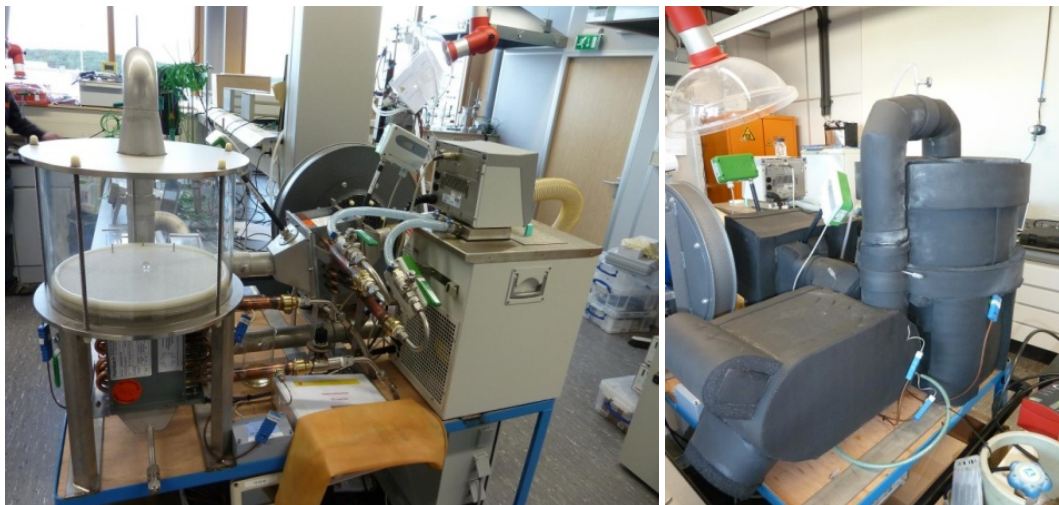
Figure 6: Photographs of prototype thermochemical storage system, (a) before and (b) after insulation.
