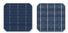
**Fig. 1** Image of n-type MWT silicon solar cells with a H-pattern based unit cell design: front side (left) and rear side (right).
