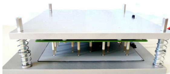
Figure 10: Chuck for applying current through an MWT-cell. The sunny side of the cell is placed on the isolated bottom plate as the measurement should be done in the dark.
