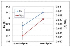
Figure 3: gain in Isc and Voc for stencil print
