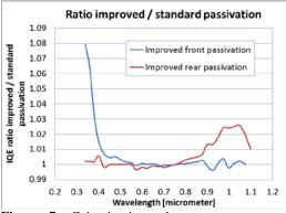
**Figure 7:** Gain in internal quantum response for improved passivation at the front (blue line) at 350 nm and at the rear (red line) between 900 and 1100 nm
