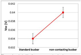
Figure 4: gain in Voc for non-contacting busbar
