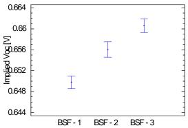
$\label{eq:states} \begin{array}{l} \mbox{Figure 5: Implied $V_{oc}$ for cells with 3 different BSF profiles with increasing sheet resistivity. ($R_{sheet\_BSF1} < $R_{sheet\_BSF2} < $R_{sheet\_BSF3}$)} \end{array}$
