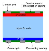
**Figure 1.** Cross section of the ECN n-pasha cell. Yingli's PANDA cells are based on this structure.
