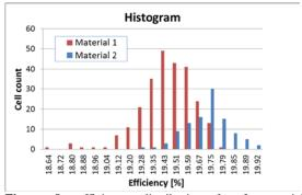
**Figure 8:** efficiency distribution for 2 materials processed with the improved n-pasha process
