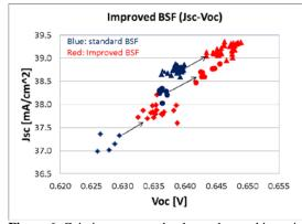
**Figure 6**: Gain in current and voltage observed in various runs using different base materials. The colors depict the type of BSF, blue for standard (BSF-1 in Figure 5) and red for improved BSF (BSF-3 in Figure 5). The symbols depict the various runs and materials used. The arrows are a guide to the eye, indicating the gain within an experiment.
