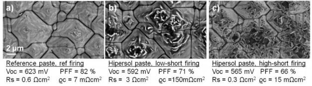
**Figure 2.** Solar cell parameters resulting from the contact microstructures shown by SEM after full contact etch, exposing the Si surface and imprints of etched-away Ag-crystallites.
