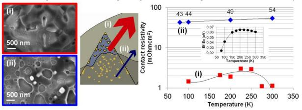
**Figure 4.** Temperature-dependent contact resistivity measurement on two different solar cell cut-outs featuring as visible by SEM after selective contact etch-back (i) direct Ag-crystallite/Ag-finger contacts, (ii) indirect contacts to Ag-crystallites through a separating glass layer. The schema shows the major current transport paths in these two samples.
