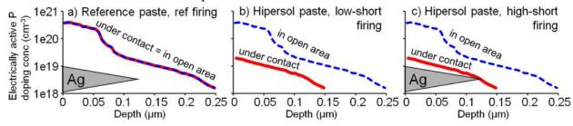
**Figure 3.** Emitter doping profile in the open-area and exemplarily under the contact including schematically an example of depth-relation to grown-in Ag-crystallites.
