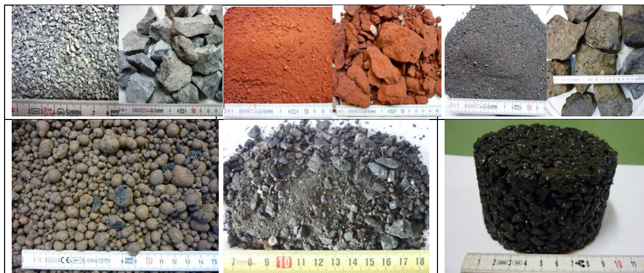
Figure 1. Some of the materials tested. Upper row from left to right: Phosphorous slag, masonry, steel slag. Lower row from left to right: Expanded clay, reclaimed asphalt, porous asphalt. Photo: BAM.
