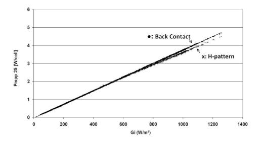
Figure 6. Temperature corrected maximum power output per cell as function of the irradiance of the back contact and H-pattern module (June 2010)
