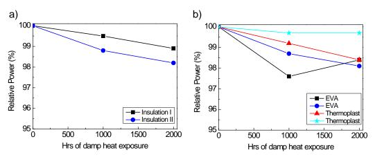
Figure 4. Relative power of MWT modules as a function of damp heat exposure. a) MWT back contact modules comprised of thermoplastic and back sheet foil with insulation coating b) MWT back contact modules comprised of either EVA or thermoplastic and back sheet foil without insulation coating.
