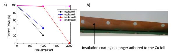
Figure 3. a) relative power of MWT back contact modules comprised of EVA and back sheet foil with insulation coating, as a function of damp heat exposure, up to 2000 hrs (2xIEC) b) photographic image of an MWT module opened after 2000 hrs of damp heat testing. The insulation coating is no longer attached to the Cu foil.
