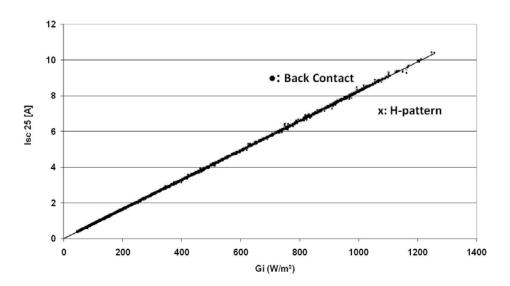
Figure 5. Temperature corrected short circuit current as function of the irradiance of the back contact and H-pattern module (June 2010).
