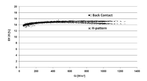
Figure 7. Temperature corrected efficiency (aperture area) as function of the irradiance of the back contact and H-pattern module (June 2010)
