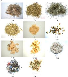
**Figure 1:** Tested types of biomass (bagasse<sup>i</sup>, grass seed hay<sup>ii</sup>, road side grass<sup>iii</sup>, straw<sup>iv</sup>, pine<sup>v-vii</sup> and spruce<sup>viii-ix</sup>) and waste streams (RDF<sup>x</sup> and Trockenstabilat<sup>xi</sup>)
