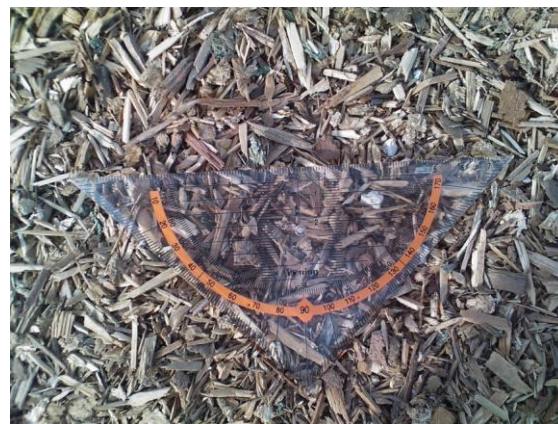
Figure 3: Demolition wood B as tested in the MILENA pilot plant
