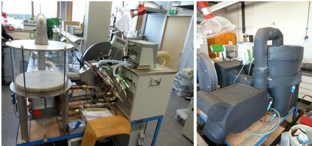
Figure 10: Photographs new prototype reactor system, (a) before and (b) after insulation.
