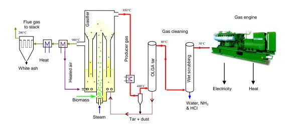
Figure 2: Basic layout of MILENA Bio-CHP plant.
