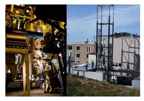
Figure 4: Pilot-scale MILENA gasifier (left) and installation of the OLGA pilot-scale gas cleaning (right).
