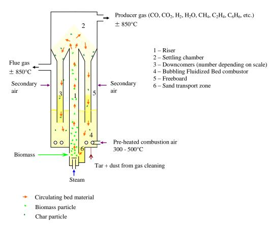
Figure 1: Simplified scheme of MILENA gasifier.
