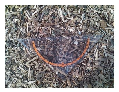
Figure 5: Demolition wood B as tested in the MILENA pilot plant.
