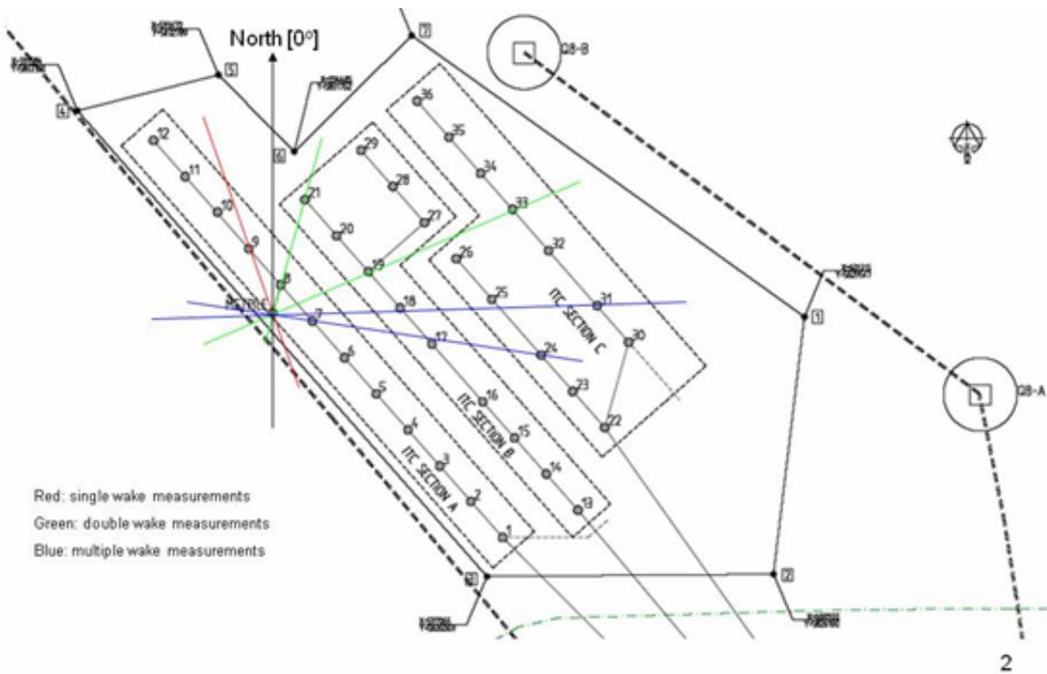
Figure 3: The lay-out of the Offshore Wind farm Egmond aan Zee (OWEZ) with wake indication. The wind farm consists of Vestas V90 turbines.
