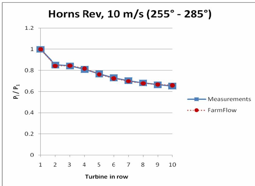
Figure 2. The power levels relative to the first turbine in the row is plotted for the sector of 255-285°.
