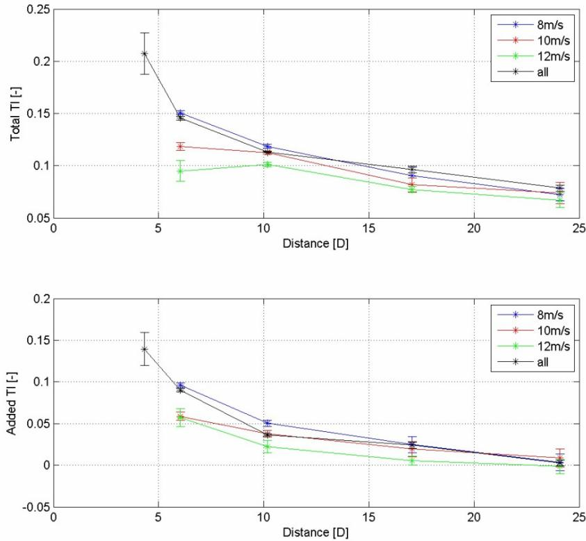
Figure 5: The measured turbulence levels at the metmast for various distances to the turbines. The upper plot indicates the measured turbulence intensity, the lower plot indicates the added turbulence due to the presence of the wake. The colors indicate wind speed intervals.
