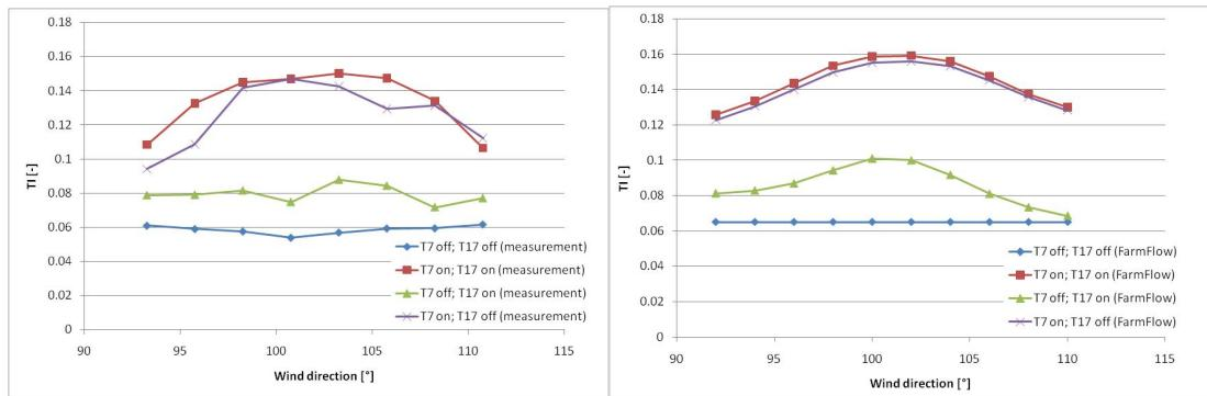
Figure 6: The measured turbulence levels at the metmast for the sector 90-110 degrees, where T7 and T17 are either operational or not. Left are measurements, right are results from Farm-Flow.
