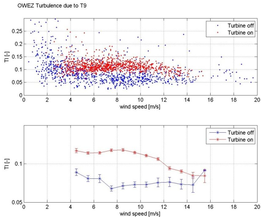
Figure 4: The measured turbulence levels at the metmast when turbine was on compared to turbine off. A limited dependency on wind speed has been observed.
