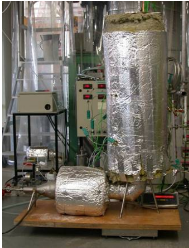
20 l batch reactor
