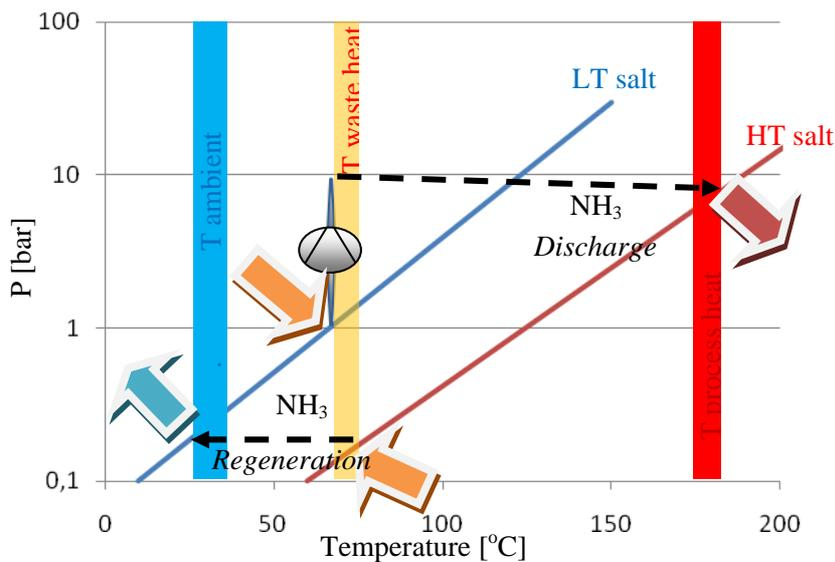
**Figure 2. Schematic diagram of a hybrid adsorption - compression heat pump for upgrading (industrial) heat to a higher temperature. The blue and red line show the sorption line of respectively low and high temperature sorbent. The colored arrows show heat flows into (at middle temperature) and out (at ambient and high temperature) of the system.**
