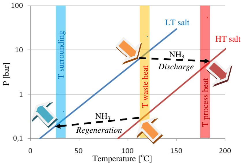
**Figure 1. Schematic diagram of a heat-driven heat pump type II for upgrading (industrial) heat to a higher temperature. The blue and red line show the sorption line of respectively low and high temperature sorbent. The colored arrows show heat flows into (at middle temperature) and out (at ambient and high temperature) of the system.**
