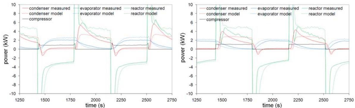
**Figure 9. Measured and calculated powers as a function of time for hybrid heat pump operation with the compressor placed between evaporator and sorption reactor (left: config 3) and placed between sorption reactor and condenser (right: config 4).**
