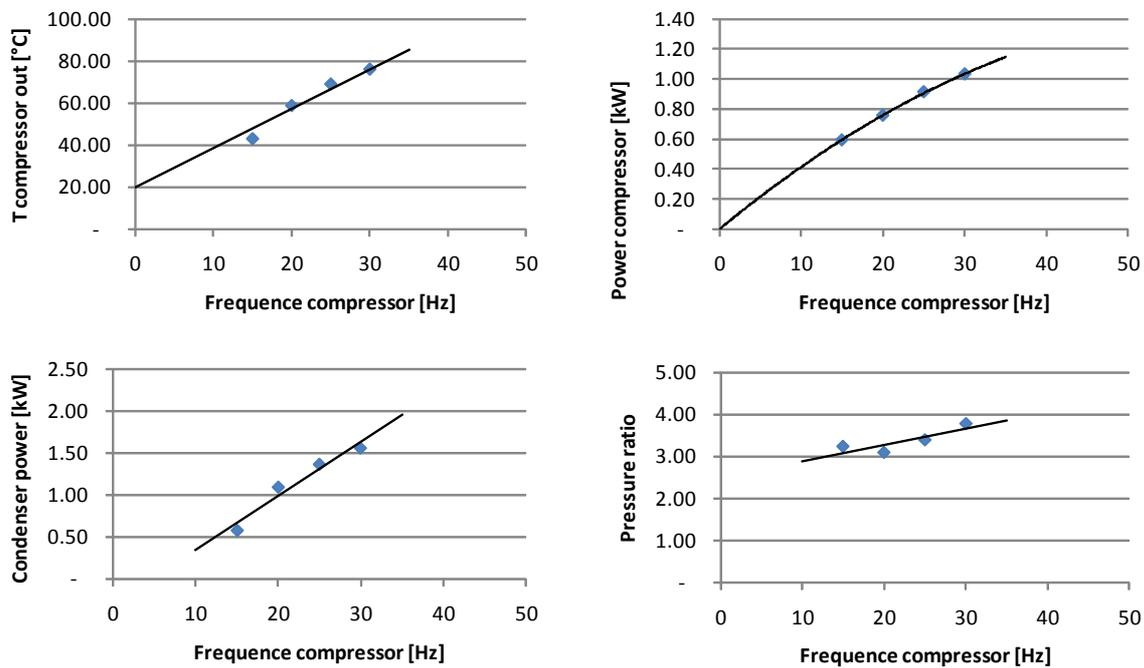
**Figure 4.** The compressed gas temperature, compressor power, condenser power and pressure ratio as a function of the compressor frequency for condenser and evaporator temperatures of respectively 20°C and 10°C.
