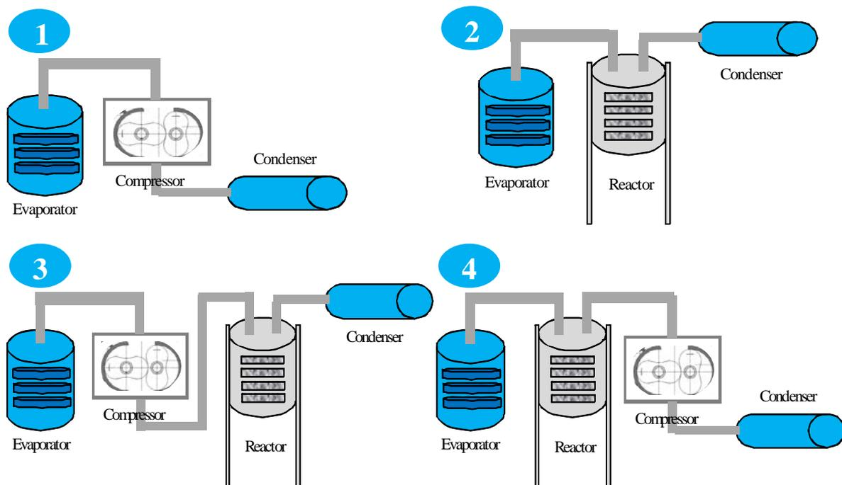
**Figure 3. The four configurations for measuring system performance: 1 - continuous 'standard' compression, 2 - purely heat-driven sorption system, 3 - hybrid system with compression at low pressure and 4 – hybrid system with compression at high pressure.**
