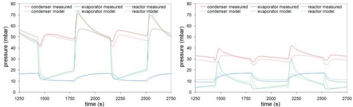
**Figure 8. Measured and calculated pressures as a function of time for hybrid heat pump operation with the compressor placed between evaporator and sorption reactor (left: config 3) and placed between sorption reactor and condenser (right: config 4).**
