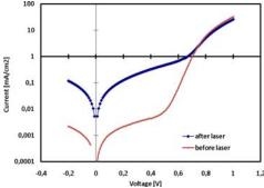
**Figure 3:** I-V curve under illumination (top) and dark (bottom) before and after laser scribing a P1 line.
