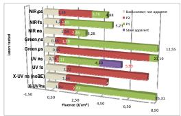
**Figure 2:** Ablation thresholds and process windows for nine different lasers on the ECN full stack sample.
