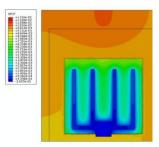
Figure 7: Example of first trial run modelling test grids using a finite elements software showing the potential distribution.
