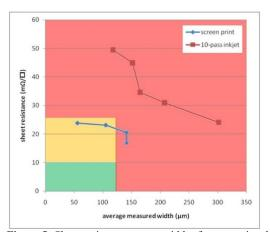
**Figure 5:** Sheet resistance versus width of screen printed and 10-pass inkjet printed lines. The red, orange and green areas indicate ideal, acceptable and insufficient performance as determined from PV specifications.
