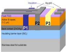
Figure 1: ECN TF-Si module concept.
