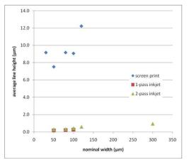
**Figure 4:** Comparison of screen printed and single and double-pass inkjet-printed metallisation on glass.
