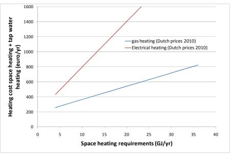
Figure 1: Annual energy cost for heating (space heating and tap water heating). For tap water heating, a fixed demand of 9 GJ/year is assumed.
