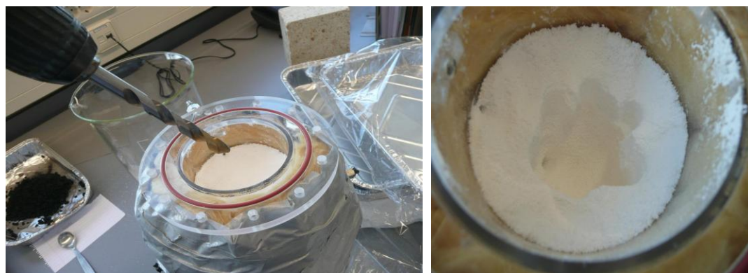
Figure 5: (a, b) Formation of a hard impregnable layer due to overhydration in open sorption reactor.
