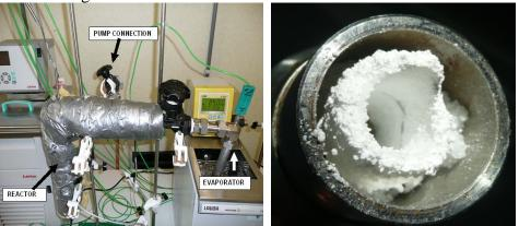
Figure 3: (a) Evacuated setup, (b) Overhydration of the magnesium chloride in the evacuated setup.
