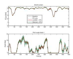
Figure 6: Power production and pitch angle in a simulation with 11 m/s wind, with distributed control options
