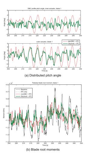
Figure 7: Results for part of the time series of a simulation with 11 m/s wind, with distributed control options
