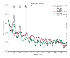
Figure 5: Spectrum for 15 m/s wind with distributed control options
