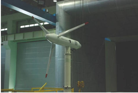
Figure 6: KARI wind tunnel with scaled down model of Mexico rotor (compare with figure 1)
