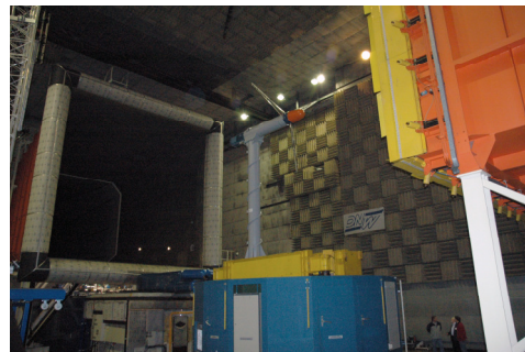
Figure 1: Set-up of the Mexico model in the LLF tunnel of DNW. The collector is shown in the background and the nozzle in the foreground
