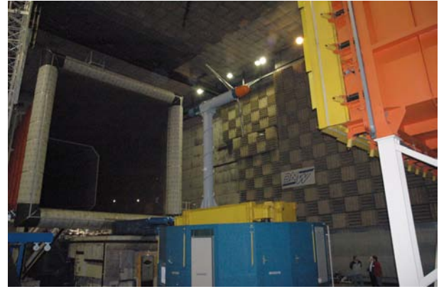
Figure 2: Setup of model turbine in the Measurement Section of the DNW LLF
