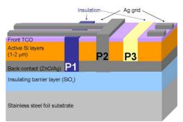
Figure 6. Thin-film silicon PV Module concept on electrically insulated steel foil substrate.
