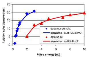
Figure 7. Ablation diameter versus pulse energy for the back contact and the  $\mu$ c-Si layer. Fitting of these curves yields the ablation thresholds of the corresponding layers for the 355 nm laser.
