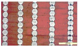
**Figure 11.** P2 scribes obtained with a 1064 nm ns pulsed laser. From left to right the spot overlap was increased.
