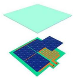
**Figure 4.** Module concept for back-contacted solar cells with low-resisitive pattern in backsheet foil, and compatibility with pick-and place technology for cell alignment.<sup>\*</sup>
