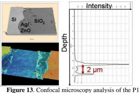
**Figure 13.** Confocal microscopy analysis of the P laser scribe.
