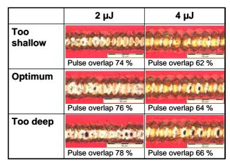
Figure 8. Pulse energy / pulse overlap combinations to achieve P2 scribes with the UV ns laser.
