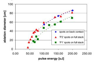
Figure 12. Diameter of ablation versus pulse energy with 1064 nm laser.
