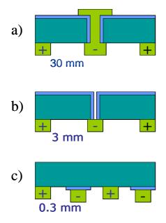
**Figure 2**. Next generations of crystalline silicon solar cells: a) metallization wrap-through (MWT), b) emitter wrap-through (EWT) and c) interdigitated back contacted cells (IBC). The typical dimensions of a 'unit cell', i.e. distance between positive and negative electrodes, is indicated.
