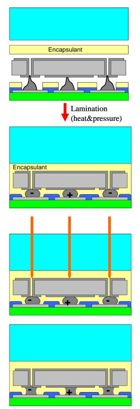
Figure 5. Process sequence for in-laminate laser soldering.
