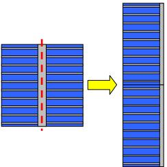
**Figure 3.** Schematic representation of cutting up an x by x H-grid pattern into a 0.5x by 2x thin film pattern. The red dashed line indicates the cutting line.
