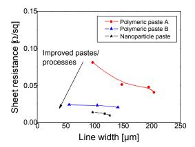
**Figure 5.** Sheet resistance of screen printed narrow silver lines from low-temperature curing pastes as function of the line width.
