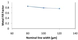
**Figure 6**. Metal fill factor for screen printed lines with polymeric paste as function of line width.
