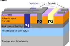
Figure 1. ECN Thin-Film-Silicon module concept.
