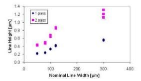
**Figure 7.** Line height as function of line width for inkjet printed lines.
