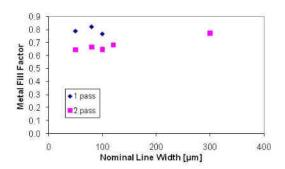
**Figure 8.** Metal fill factor as function of line width for inkjet printed lines.
