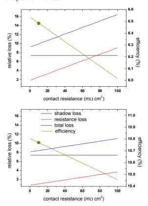
**Figure 4.** Calculated losses for amorphous single junction (top) and amorphous/microcrystalline tandem modules (bottom) as function of contact resistance between front TCO and printed Ag.
