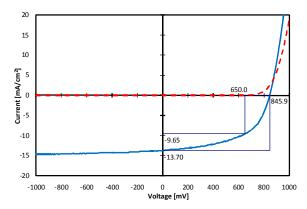
Figure 2: JV-curve of nip solar cell on a rigid substrate: Asahi U-type glass coated with a sputtered Ag/ZnO back contact.
