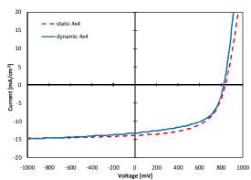
Figure 4: Comparison of JV-curves of nip solar cells on Asahi glass substrates deposited in-line (solid, blue) with those deposited in a step-roll process (dashed, red).
