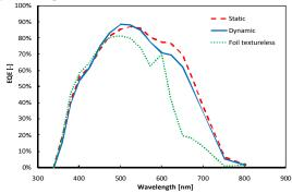
**Figure 6**: EQE curves of the presented solar cells: step-roll (dashed, red), in-line on rigid substrate (solid, blue) and inline on flexible, texture-less substrate (dotted, green).
