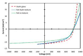
Figure 5: JV-curve of nip solar cell deposited on steel foil coated with Asahi-textured barrier layer and Ag/ZnO back contact compared with nip solar cell deposited on Asahi glass (dashed, red). Flexible cells with Asahi-textured barrier layer and flat barrier layer are shown, respectively as solid blue and dotted green lines.
