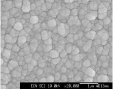
Figure 3: SEM picture of an Asahi U texture (top) and the ITO surface of a nip solar cell grown on Asahi-U glass substrate coated with a sputtered Ag/ZnO back contact (bottom).
