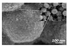
Figure 2. SEM pictures of TiO<sub>2</sub> beads
