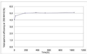
**Figure 6.** Temporal evolution of the active area efficiency measured at  $250~\text{W/m}^2$  of Swerea modules upon continuous exposure to  $1000~\text{W/m}^2$  light at approx.  $50~^{\circ}\text{C}$ . Dye: C101; Electrolyte: 1~M 1,3-dimethyl Imidazolium iodide, 0.5~M N-butylbenzimidazole, 0.15~M I<sub>2</sub>, 0.1~M Guanidinumthiocyanate in Methoxypropionitrile
