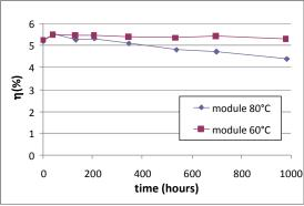
**Figure 5.** Temporal evolution of the active area efficiency of ECN modules upon exposure to 60 and 80 °C in the dark. Dye: C101; Electrolyte: 0.6 M Propyl-Methyl-Imidazolium Iodide, 0.1 M I<sub>2</sub>, 0.5 M N-methyl-Benzimidazole in Propionitrile.
