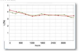
**Figure 7.** Temporal evolution of the efficiency measured at 1000 W/m² of a 3Gsolar cell upon continuous exposure to 85°C Dye: C101(red line), N719 (green line); Electrolyte: Dyesol HSE (high stable electrolyte).
