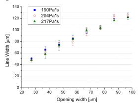
**Figure 5:** Printed line width as a function of stencil opening width for 3 different viscosities
