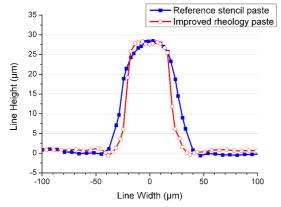
**Figure 7**: Cross section comparison of reference stencil paste and improved rheology paste printed through a 60μm opening in a 50μm thick stencil
