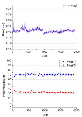
Figure 10: Line resistance, line width and height as a function of cell number
