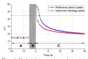
**Figure 6:** Rheological time test showing loss angle as function of time in the three intervals.
