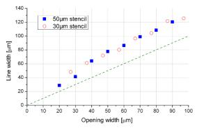
**Figure 2:** Printed line width as function of stencil opening width for  $50\mu m$  and  $30\mu m$  thick stencil,. Dashed line gives line width without spreading
