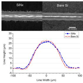
**Figure 3:** Top views and cross sections of a finger deposited on SiNx, and on bare Si
