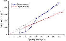
Figure 1: Line cross sectional area as a function of stencil opening width for a  $50\mu m$  and a  $30\mu m$  thick stencil
