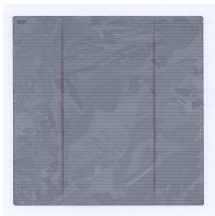
Figure 3: A wafer with an H-pattern selective emitter after diffusion, before PSG removal.
