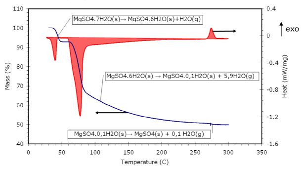
Figure 2: A typical TG-DSC curve for dehydration of MgSO<sub>4</sub>.7H<sub>2</sub>O. A sample of 10 mg is heated up from 25°C to 300°C with 1°C/min. During the experiments a N<sub>2</sub>+H<sub>2</sub>O gas mixture was used with PH2O~2.1 kPa. The blue line denotes TG curve and the red line denotes the DSC curve.
