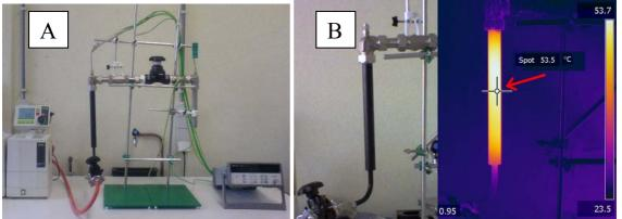
Figure 4: Experimental Set-up (a) set-up, (b) close-up of reactor vessel (normal photograph and infrared photograph showing the reaction temperature for hydration of zeolite)
