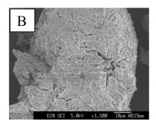
Figure 3: SEM images of magnesium sulfate particles (38-106  $\mu$ m): A; before dehydration (15 kV, x500 magnification), B; after dehydration (5 kV, x1500 magnification).
