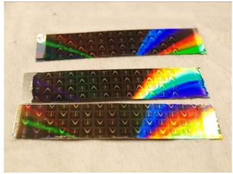
Fig. 7: First nip a-Si solar cells on steel foil + barrier layer + periodic texture.
