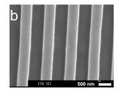
Fig. 4 SEM images of a metal master with a 1000 nm period grating (a) and its replica in the sol-gel barrier layer (b). The scale bar in both images represents 100 nm.
