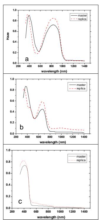
Fig 5. Haze measurements on master and replicas with diffraction gratings of (a) 1000 nm, (b) 750 nm, and (c) 500 nm.
