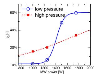
Fig. 6: Crystalline fraction of microcrystalline silicon layers, as a function of the applied microwave power.
