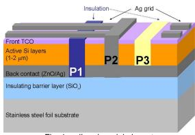
Fig. 1: cell and module layout
