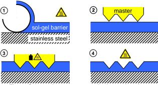
Fig. 2: Schematic process steps for hot embossing.
