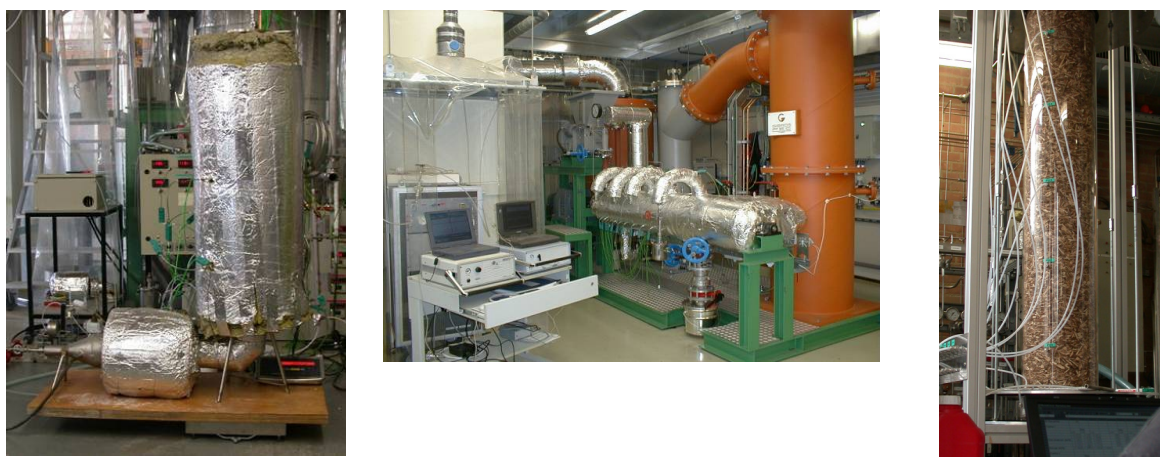
Figure 3: Equipment for bench-scale testing: 5 liter batch reactor (left), 5 kg/h Auger (screw) reactor (middle) and cold flow reactor (right)
