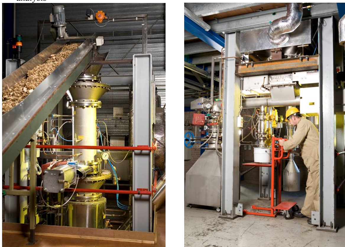
Figure 6 Biomass being fed to the top section of the pilot plant (left) and bottom section of the pilot-plant (right) (Photos Jasper Lensselink)
