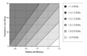
Figure 2: Iso-cost curve for Advanced Basepower technology regarding cell efficiency and feedstock cost.
