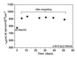
**Figure 4:** investigation of lifetime stability of deposited a-Si:H(p).
