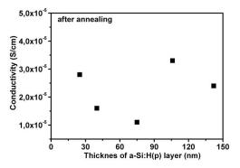
**Figure 2:** surface recombination velocity of annealed a-Si:H(p) layers as function of layer thickness (upper); dark conductivity obtained for the same a-Si:H(p) layers as function of layer thickness (lower).
