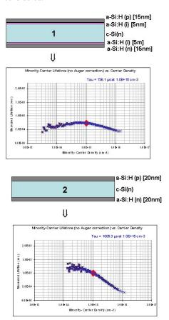
**Figure 6:** schematic drawing of stack layer 1 and corresponding minority charge carrier lifetime (upper); schematic drawing of stack layer 2 and corresponding minority charge carrier lifetime (lower).
