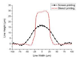
**Figure 6:** Finger profile comparison between stencil (60μm) and screen (105μm opening)
