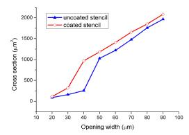
**Figure 5:** Cross section as function of opening width for coated and uncoated stencils
