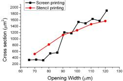
Figure 2: Cross section as function of opening width for stencil and dual layer stencil
