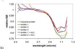
**Figure 6:** IQE profiles relative to cells from comparable heights of the reference ingot. a) ingot height dependence for the 10% (blue) and 25% (yellow/brown) SOLSILC blends, processed with emitter 3 (and no clean). b) different emitters with and without extra cleaning step.
