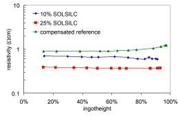
Figure 1: Resistivity profiles of the multicrystalline ingots measured by inductively coupled coil measurements.
