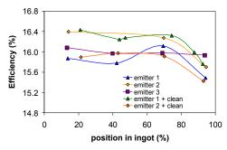
**Figure 5:** Conversion efficiency of the blended ingot with 25% SOLSILC Si against position in the ingot for all 5 optimized processes. The wafer positions refer to the full height of the ingot (including bottom and top pieces that are usually cut off).
