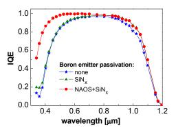
Figure 7: Internal quantum efficiency of cells with and without wet chemical oxide (NAOS).
