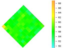
**Figure 6**: Sheet resistance mapping of a 60  $\Omega$ /sq boron emitter.
