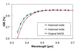
**Figure 8**: Internal quantum efficiency of cell with original NAOS oxide passivation and IQE of two cells with improved wet chemical oxidation.
