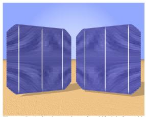
**Figure 5**: Artist impression of a bifacial front-side junction cell.
