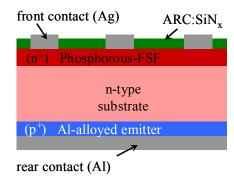
Figure 1: Cross section of rear-side junction n-type cell.
