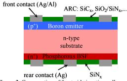
Figure 3: Cross section of front-side junction cell.
