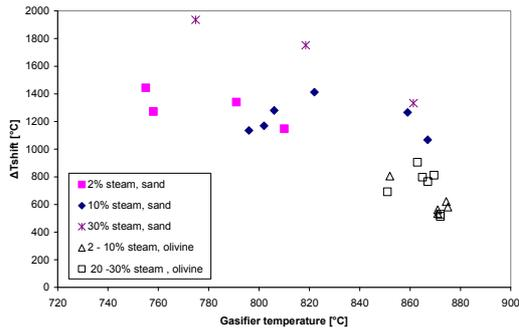
Figure 2: Effect of temperature on CO shift equilibrium
