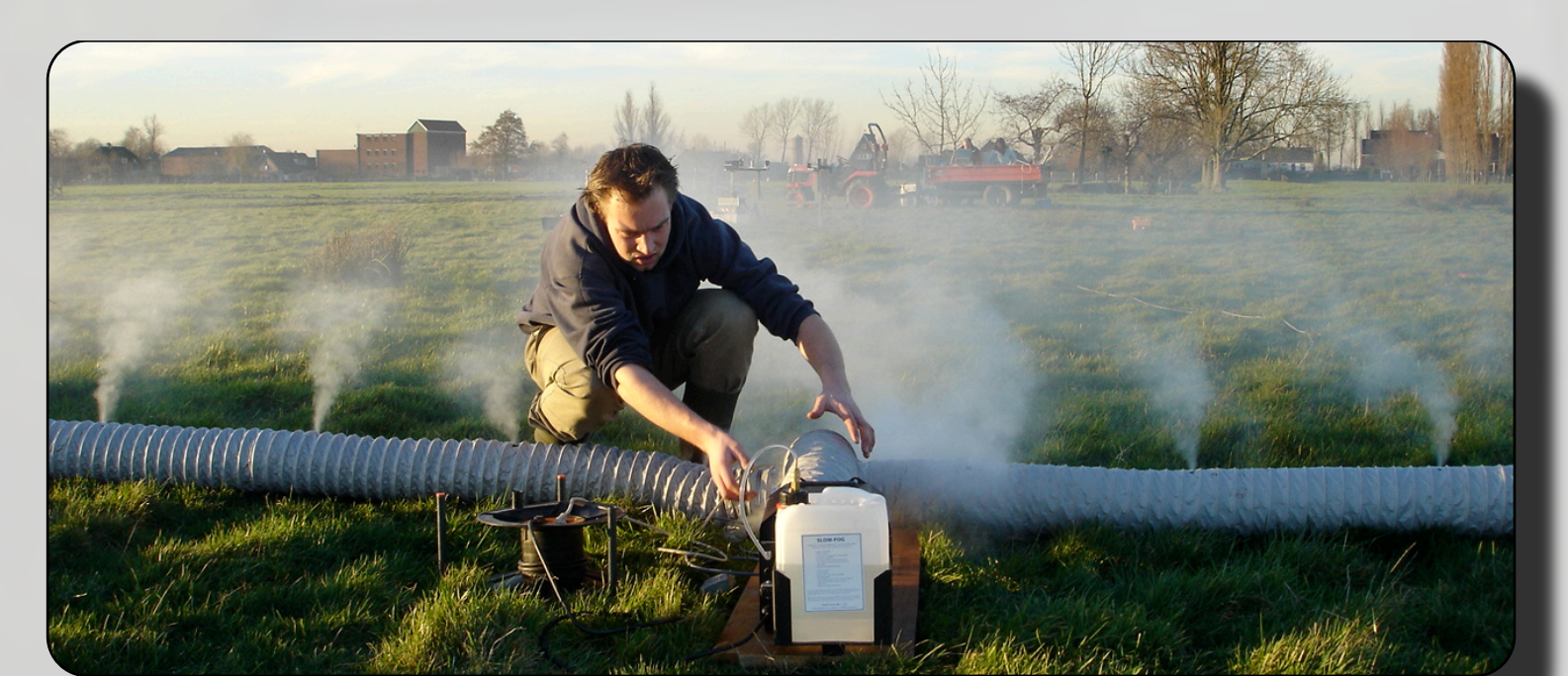
Seeding system: conventional smoke-machine
